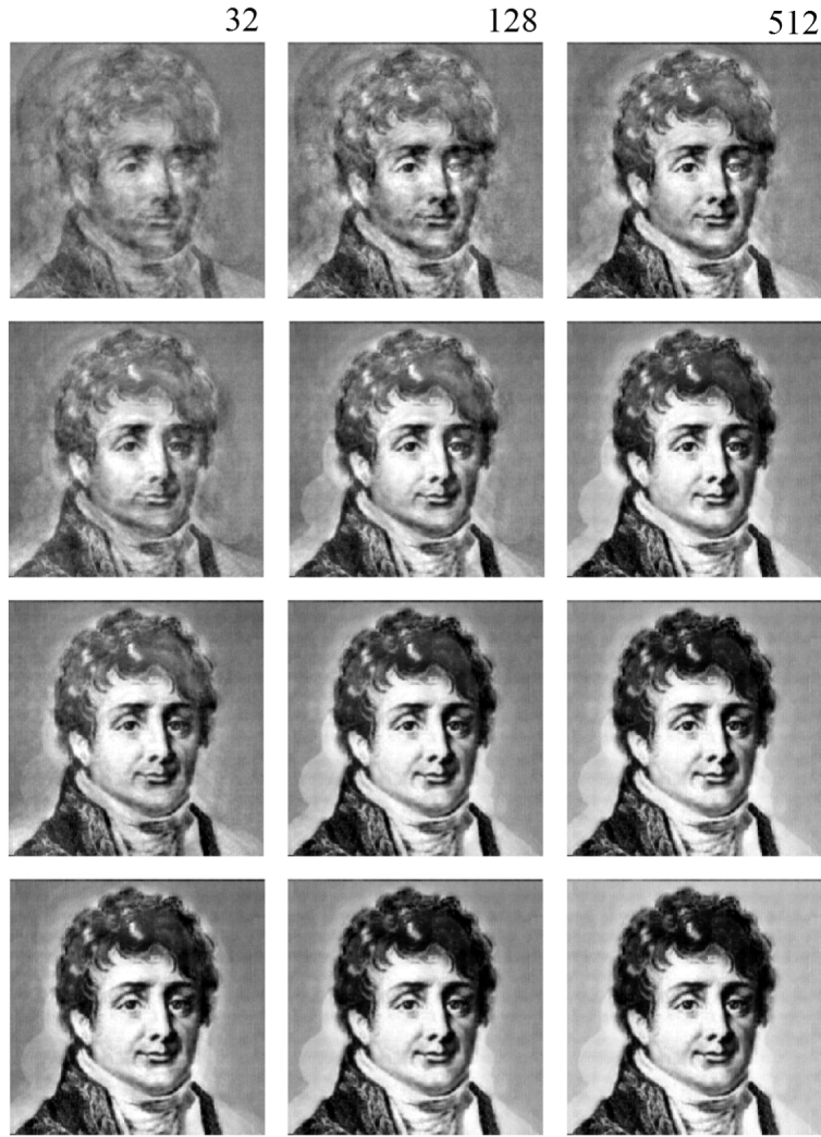
FIGURE 13.31: Associative memory convergence using Fourier using the library of pictures in Figure 13.27 and 13.28. The greater the percentage (1%, 4% 9%, 16%) of the known image, the faster the convergence. An error curve is shown in Figure 13.32.
