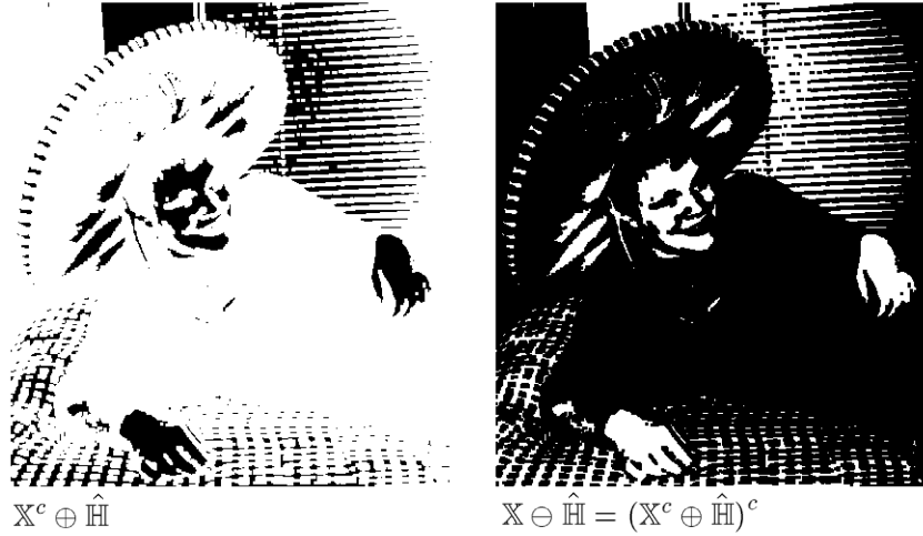
FIGURE 14.27: Illustration of the erosion duality theorem in (14.52). The pictures corresponding to \mathbb{X} and \mathbb{X}^c are shown in the top row of Figure 14.26.
