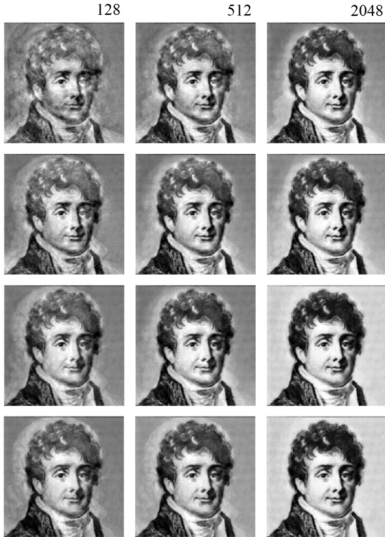
FIGURE 13.34: Convergence of the POCS associative memory as a function of the library size. The convergence of Fourier for 56, 28, 14 and 7 library vectors is shown. In each case, the Fourier is included in the library. A plot of error is shown in the next figure (Figure 13.35). The larger the library, the slower the convergence.
