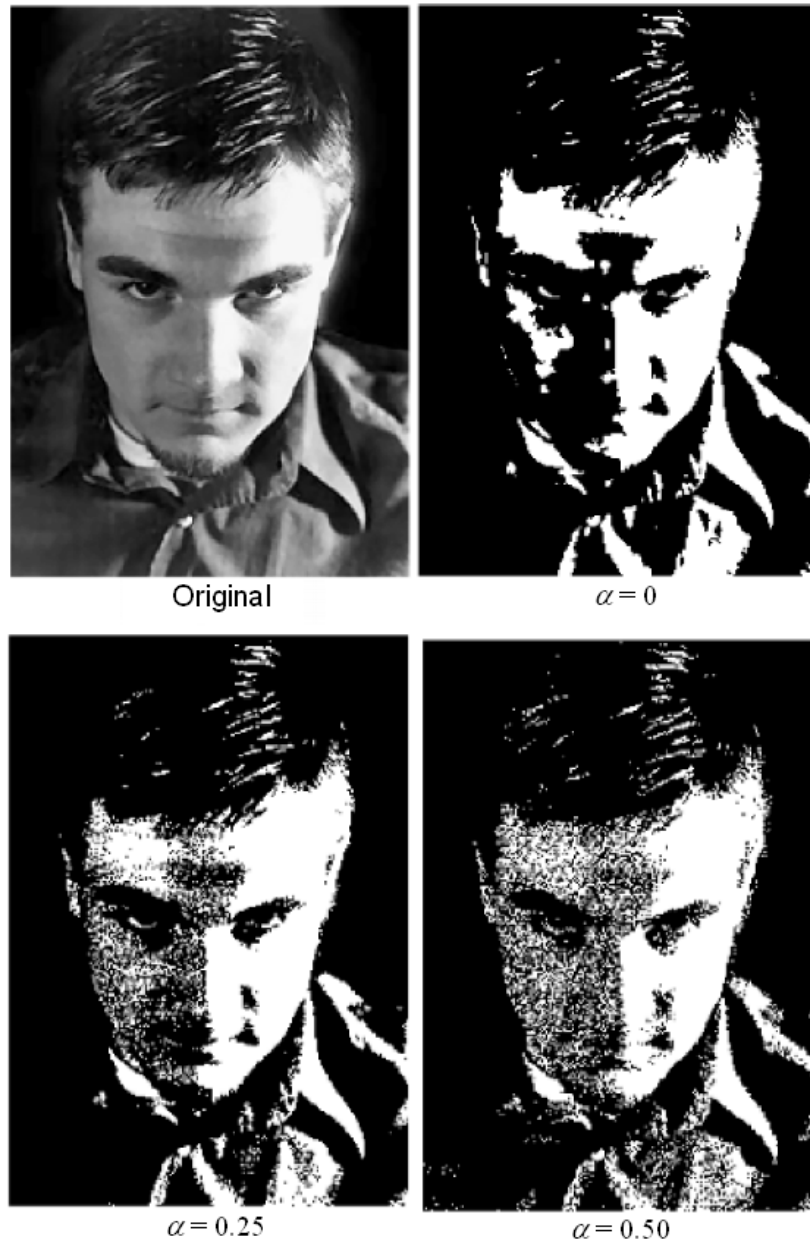
FIGURE 5.13: (Continued in Figure 5.14.) An example of stochastic resonance. The picture, Jeremiah , at the upper left is subjected to additive noise in (5.53) for various values of \alpha and is then thresholded at the mid of the gray scale range. Values greater than 1 are pictured as white and those below zero are set to zero. The \alpha = 0 image is simply the original image thresholded. The \alpha = 0 corresponds to too little noise and \alpha = 1.75 is too much. The optimal amount of noise, corresponding to stochastic resonance , lies somewhere in between. As shown in (5.54), \alpha = 0.5 gives the best stochastic representation of the original image.
