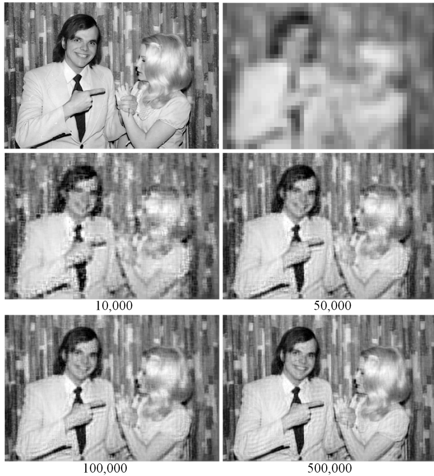
FIGURE 13.58: Subpixel resolution using POCS and the constant area convex set. After a half million projections, the image at the bottom left resembles the original image at the upper left.
