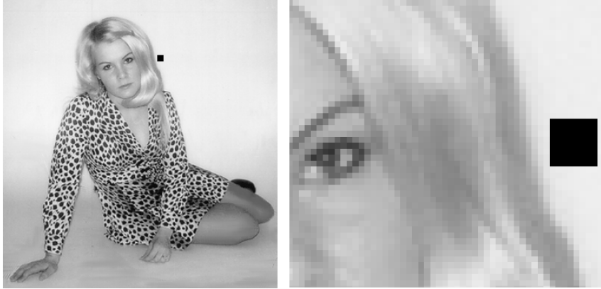
FIGURE 9.43: An 8 \times 8 block of pixels in this 345 \times 363 pixel is shown on the left as black square. A zoomed version of the image is shown on the right.
