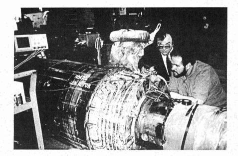
Shorted turns in the field winding of large turbogenerators (2 or 4 poles) are a common problem whose detection and localization have remained elusive. Shorts occur primarily from incessant pounding of the rotor copper conductors while the machine is turning in low gear. This low speed operation is designed to avoid the deformation of the shaft that occurs when the rotor remains stationary in the bore for long periods of time.
