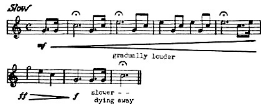
Figure 2: Taps is played with four notes. They are the 3 rd through 6 th harmonics of the bugle’s vibrating air column.
