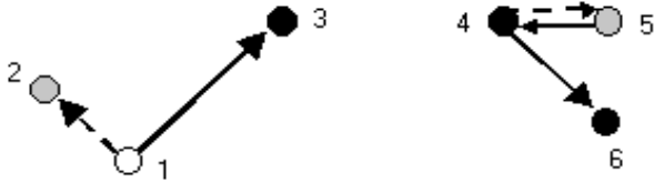
Fig. 7. The loop \{4 \leftrightarrow 5\} is formed by a combination of cost-incurring and free transmissions. As in Figure 6, The sets \{1,2,3\} and \{4,5,6\} are disjoint.
