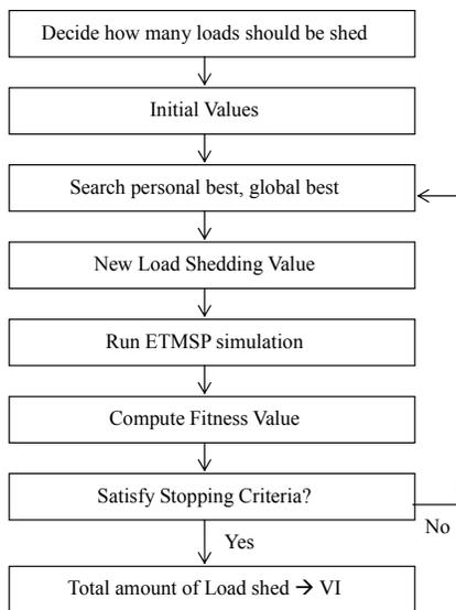
Fig. 10. The overall procedure of PSO method.
