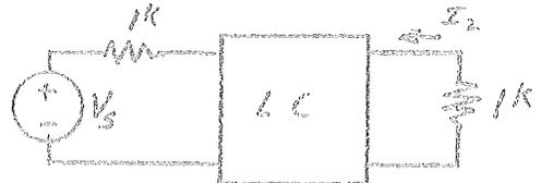
as a lossless ladder network terminated at both ends in a 1000-Ohm resistance.
