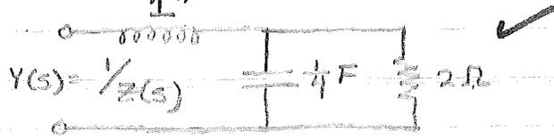
c) CHECKING DRIVING POINT IMPEDANCE
