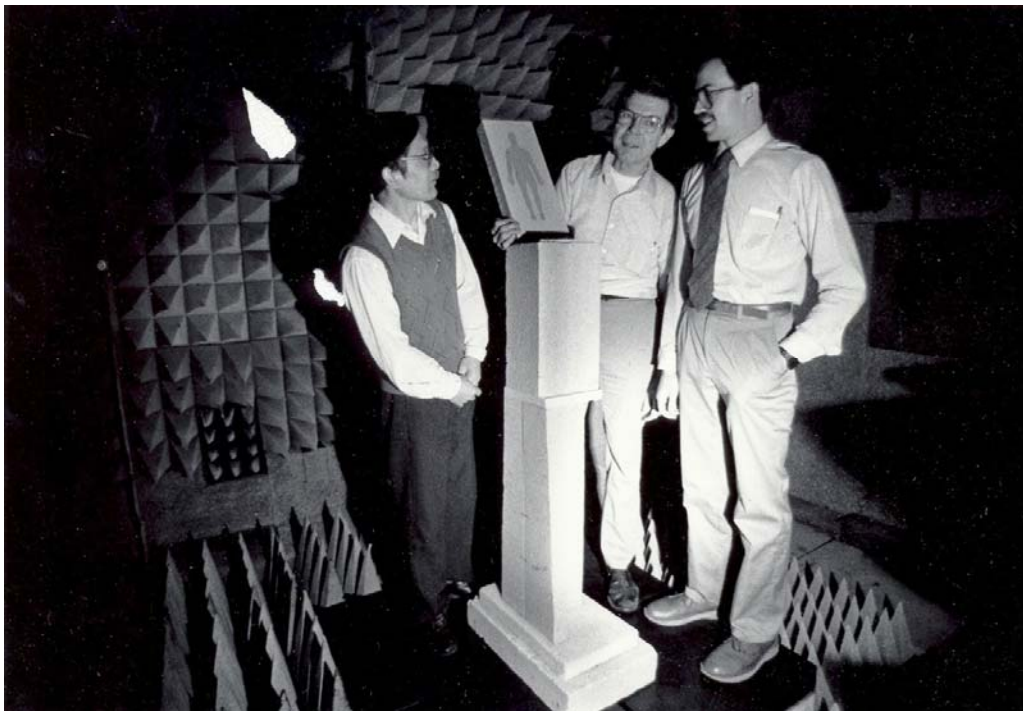
Figure 116. Anechoic chamber in the 1948 Electrical Engineering Building being used for electromagnetic exposure measurements on a scale human, ca. 1977. At center is probably Arthur Guy. The photograph has some damage. ( Trend photo)
