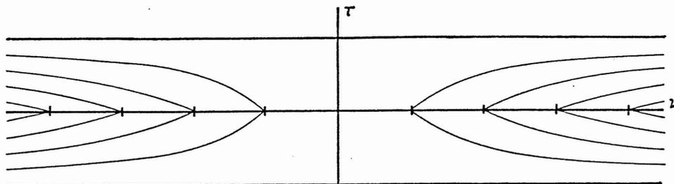
Fig. 3. Zero locus plot of the ambiguity function of a single pulse.
