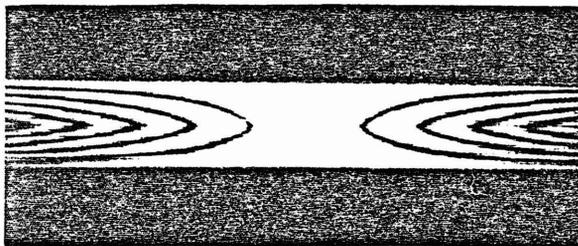
Fig. 4. The ambiguity function (modulus squared) display for a single pulse, as generated by the coherent processor of Fig. 2.
