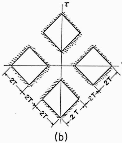
Fig. 5. (a) A double pulse. (b) The corresponding function  $f[(t + \tau)/\sqrt{2}]f[(t - \tau)/\sqrt{2}]$  in the  $(t, \tau)$  plane.
