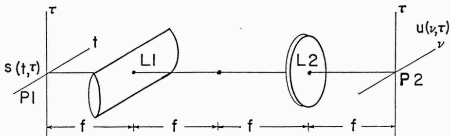
Fig. 2. A coherent processor for ambiguity function display. Both the lenses have focal length  $f$ . Fourier transformation is performed in the horizontal direction and imaging in the vertical direction.
