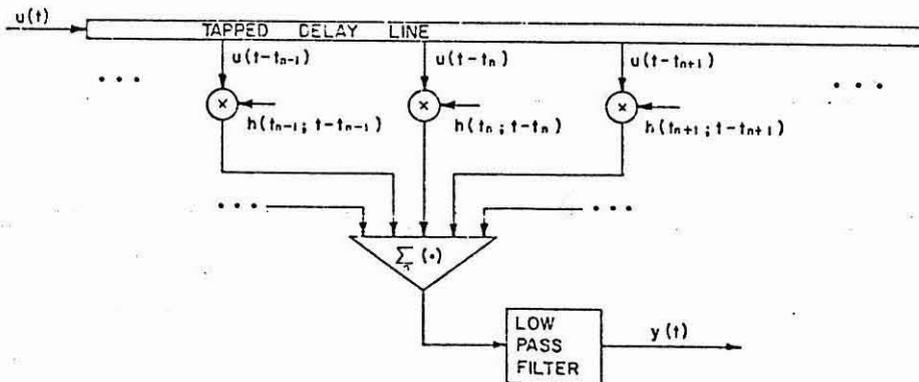
Figure 2: An implementation of the sampling theorem presented in section 5. Delayed versions of the input are multiplied by corresponding sample impulse responses, summed, and passed through a low pass filter to give the output of the parent shift variant system.
