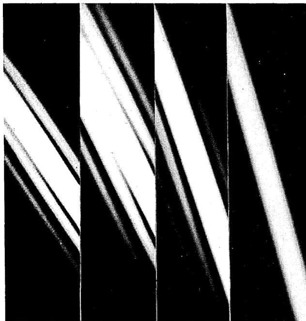
Fig. 2. Processor outputs for various unit pulse inputs. The Mellin transform appears along the vertical axis in each case.
