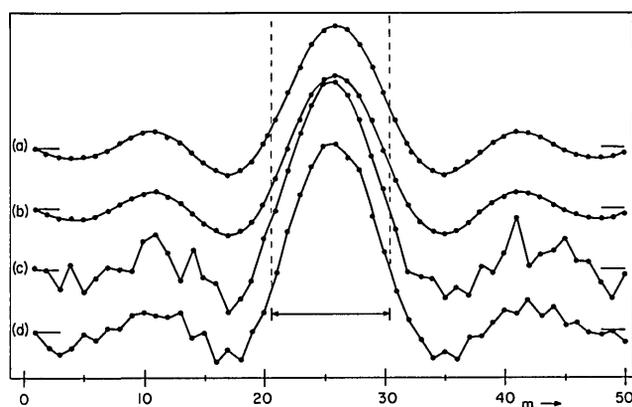
Fig. 8. Interpolation of ten points of a sinc,  $\beta = 5$ : (a) object; (b) noiseless interpolation; (c) interpolation in the presence of additive noise; and (d) filtered results.
