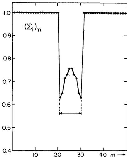
Fig. 3. Normalized noise level for interpolation,  $\beta = 3$ . The standard deviation for the ten interpolated points (within arrow) is lower than that of the data.
