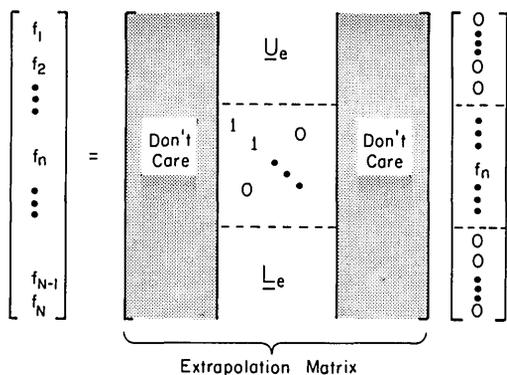
Fig. 2. Structure of the extrapolation matrix  $\mathcal{E}$ .
