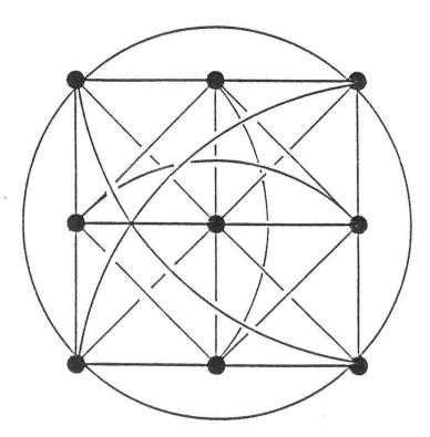
Figure 4: A LINN to solve the *Queens Problem* on a 3 by 3 chess board. Every interconnect has a value of - c.
