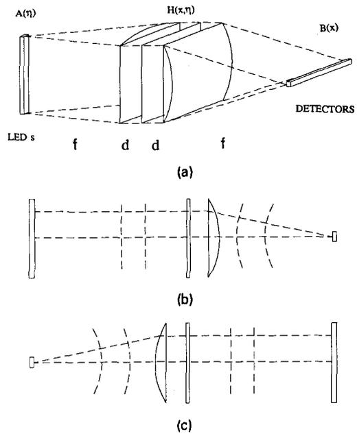
Fig. 4. (a) Diagram of a matrix-vector multiplier; (b) side view; (c) top view.
