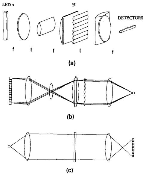
Fig. 5. (a) Illustration of the Stanford matrix-vector multiplier; (b) side view; (c) top view.
