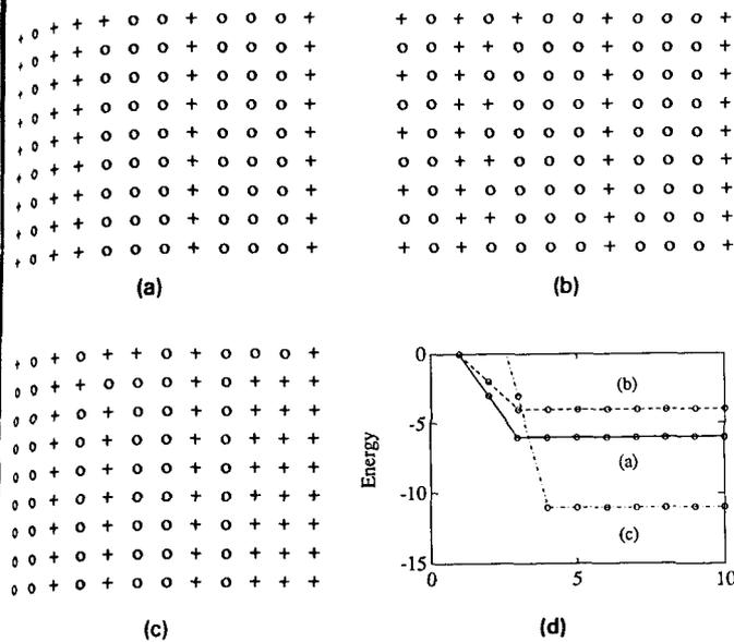
Fig. 3. Examples of stability and convergence in Hopfield's model. Iteration time in (a), (b), and (c) are in rows top to bottom (+ denotes +1). The first row is the result of the first iteration. We see that  $s(0)$  (a) converges to  $v_2$  without skew, (b) oscillates with skew, and (c) converges to a vector with a different skew that is not in the library. (d) Energy transitions with iteration for each case.
