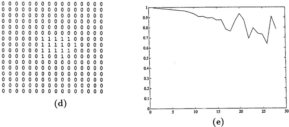
Figure 4: (a) A desired frequency response of an FSS. (b) The corresponding 2-D surface. (c) The first inverted unconstrained surface. (d) The constraints satisfied surface of (c). (e) The frequency response of the surface in (d).
