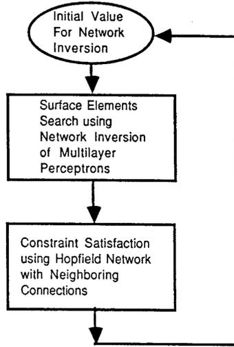
Figure 3: The schematic diagram of a complete FSS design based on iterative inversion of neural networks.
