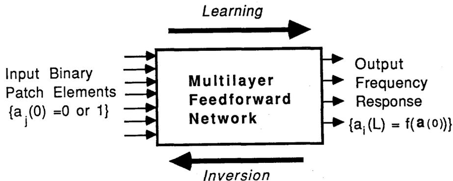
Figure 2: Learning and inversion of a multilayer perceptron.
