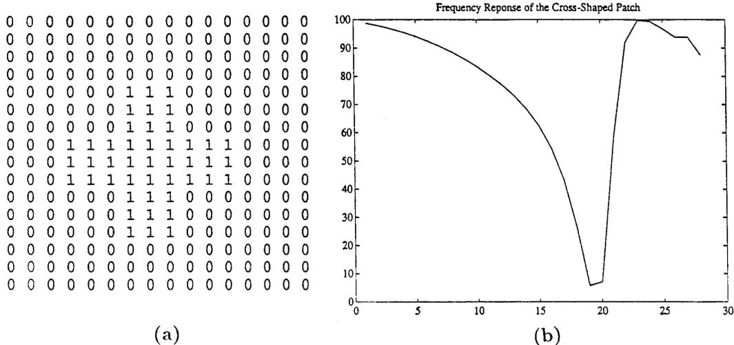
Figure 1: (a) In an FSS, subcells that correspond to the conductor region of the unit cell are represented by 1's whereas subcells outside the conductor region are represented by 0's. (b) The corresponding frequency response of the FSS.
