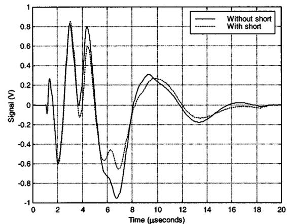
Fig. 7. Typical signature signals for stopped test rotor.
