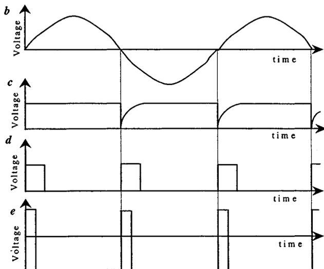
Fig. 3. Waveforms at various points in the signal generator circuit.
