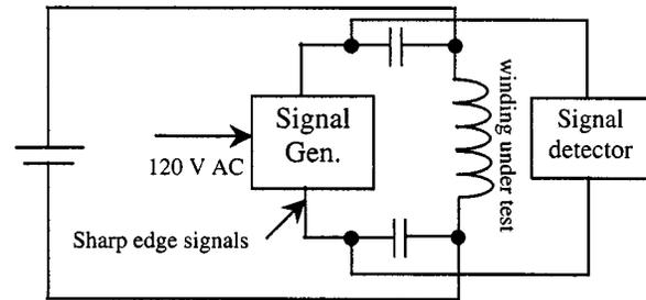
Fig. 1. Block diagram of hardware setup.
