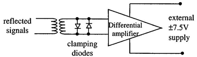
Fig. 5. Block diagram of signal detector circuit.
