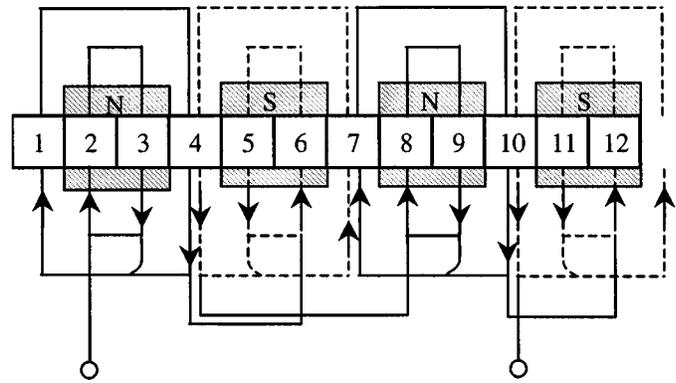
Fig. 8. Winding configuration of test rotor.
