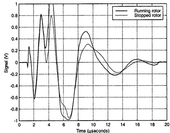
Fig. 9. Variation in signature signals due to speed of rotor (without shorts).
