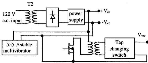
Fig. 4. Power supply circuit for signal generator.
