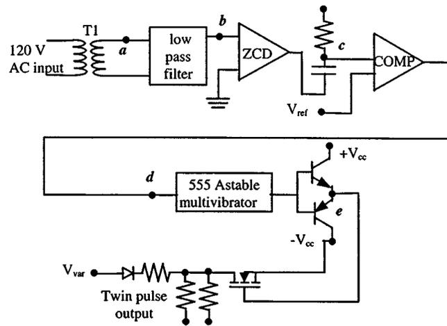
Fig. 2. Main circuit diagram of signal generator.
