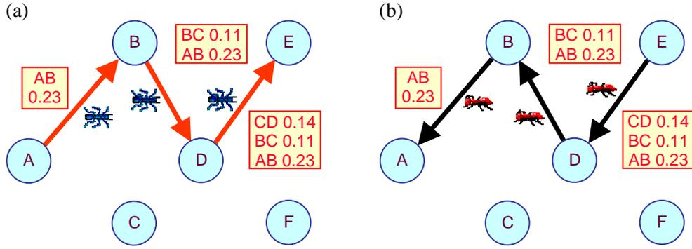
Figure 1: (a) Forward, and (b) backward ant movement in the AntNet algorithm.
