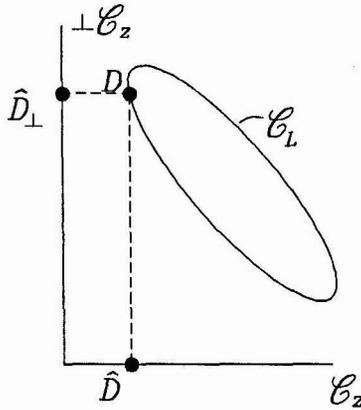
FIGURE 1: The projection of the true object,  $D$ , is the vector image  $\hat{D}$ . It is onto the column space,  $C_z$  of the matrix  $W$ . The true object,  $D$ , is also known to lie in a set of line-like objects,  $C_L$ .
