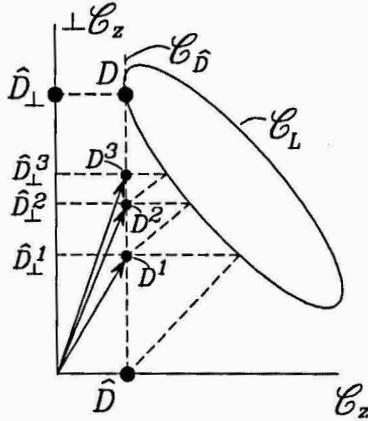
FIGURE 2: Illustration of the iterative improvements by alternating projections to reconstruct the true object  $D$ .
