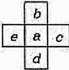
FIGURE 3: Five neighboring pixels in an image. The line-like projection is obtained by comparing the intensity of the pixel  $a$  to the intensity of the surrounding pixels  $e$ ,  $b$ ,  $c$ , and  $d$ .
