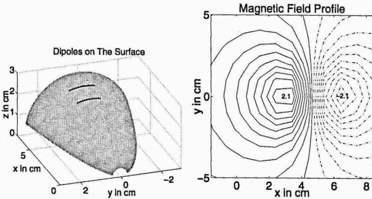
FIGURE 4: (Left) Layout of the conductors and the parabolic surface in Cartesian coordinates, (right) normal component of the magnetic field; positive contours are with solid lines and the negative contours are with dashed lines.
