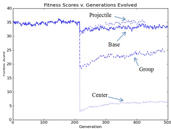
Figure 1. The results of the evolution before and after breaking the four sensors are shown here. Before generation 200, the swarm is evolving with all of its sensors. At the discontinuity, the graph splits to represent the fitness scores after the removal of the sensors. The swarm performs well with its projectile and base sensors removed and okay without its group sensor, but very poorly when the center sensor is disabled.
