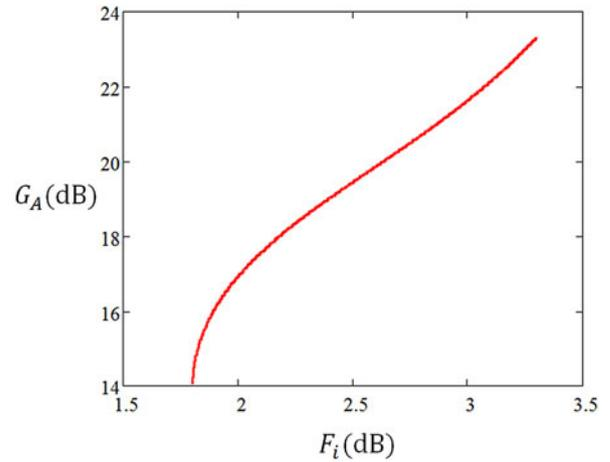
Fig. 7. Pareto front for Example 2: values of available gain  $G_A$  for different limiting values of noise figure  $F_i$ .
