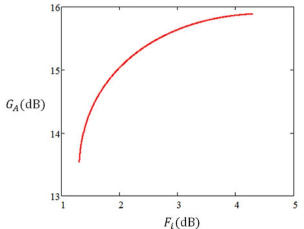
Fig. 4. Pareto front for Example 1: values of available gain  $G_A$  for different limiting values of noise figure  $F_i$ .
