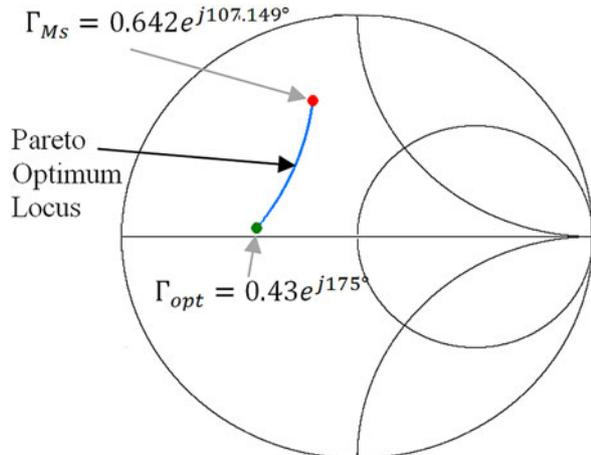
Fig. 3. Pareto optimum locus for Example 1: the collection of  $\tilde{\Gamma}_s$  points providing optimum available gain for different bounded noise figure values. Note that the Pareto locus is *not* a straight line.
