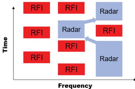
Fig. 4. Radar frequency agility to avoid interference “RFI”, reprinted from [8]
