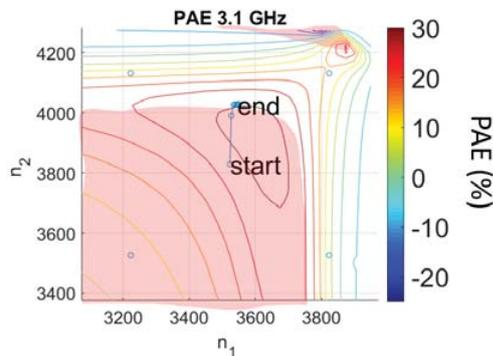
Fig. 5. 3.1 GHz search trajectory plotted atop the contours for PAE and the spectrally forbidden region (shaded). Reprinted from [6].
