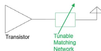
Fig. 2. A tunable matching network is placed between the transistor and antenna in each array element.
