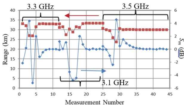
Fig. 6. Range and spectral mask compliance for the three-frequency agility experiment, reprinted from [6].
