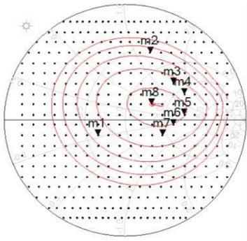
Fig. 3. Simulated output power variations based on scan-angle impedance variations presented by Allen [2]. The output power contours are in 1 dB steps. Notice that at point “m2 (text says m1)” representing an impedance for a particular value of array scan angle, the output power is approximately 3 dB below the maximum output power. This half-power loss corresponds to a 16 percent reduction in radar range.
