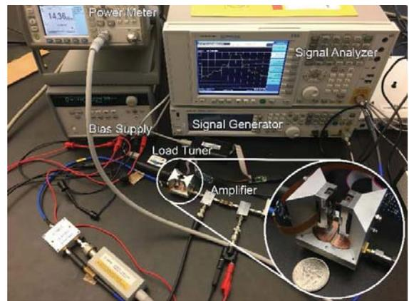
Fig. 4. Measurement setup for initial algorithm demonstration on the second-generation evanescent mode cavity tuner, reprinted from [6]
