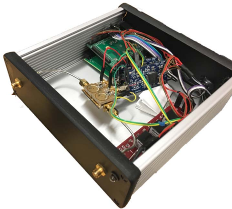
Fig. 2. 90 W EVA tuner constructed at Purdue University [4]
