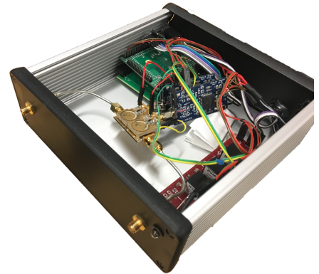
Fig. 1. Evanescent-mode cavity tuner with piezo actuators [2]
