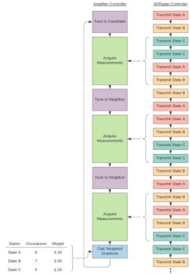
Fig. 2. Simplified example scenario of impedance tuning during relatively quickly changing transmit states.
