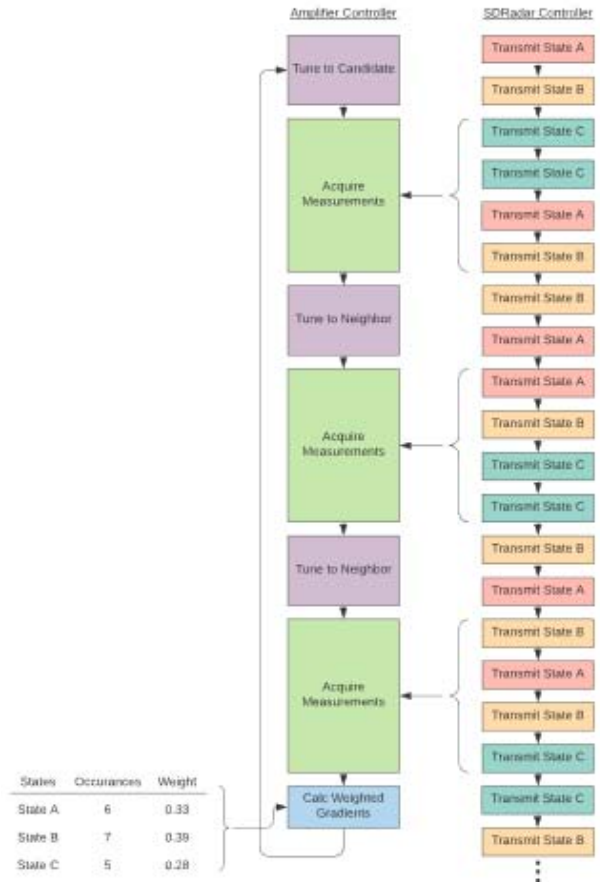
Fig. 2. Simplified example scenario of impedance tuning during relatively quickly changing transmit states.
