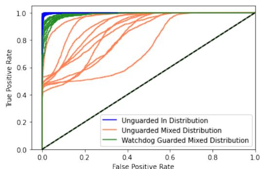
Fig. 10: The ROC plots showing the watchdog performance on the three evaluation datasets. Blue indicates unguarded in-distribution performance, Orange indicates unguarded mixed-distribution performance, and Green indicates guarded mixed-distribution performance.
