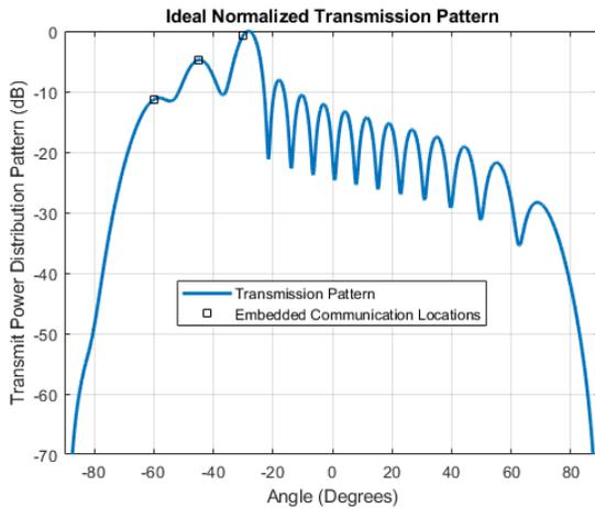
Fig. 4. Ideal directionally modulated transmission pattern, including embedded communication symbols.
