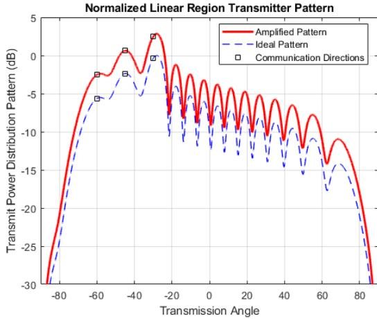
Fig. 6. Linear region transmission pattern. The amplified pattern has very good correspondence to the target transmission pattern.
