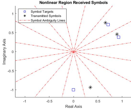
Fig. 9. Nonlinear region communication symbol integrity. In this test, one transmitted communication symbol is mistaken for another. This communication symbol is in the  $-45^\circ$  direction.
