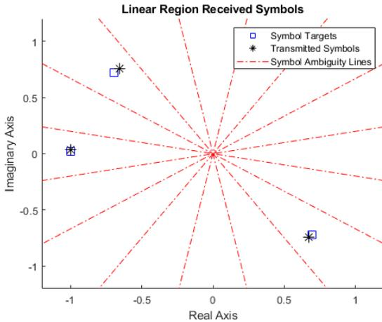
Fig. 11. Amplifier effect on the second set of communication symbols. In the linear region the communication symbols maintain integrity.
