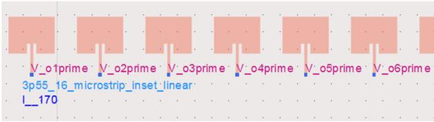
Fig. 3. Six of the 16 antenna elements used for EM simulation
