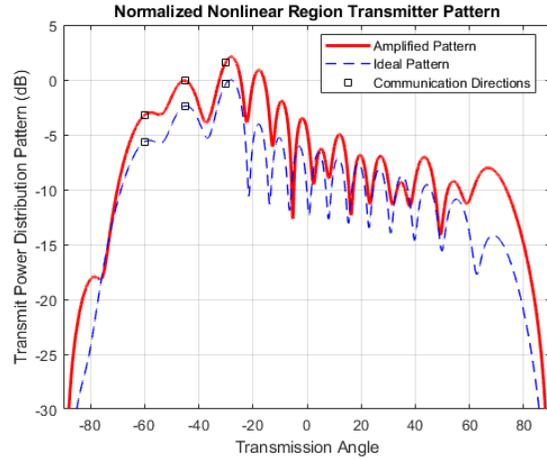
Fig. 8. Nonlinear region transmission pattern. Operation in this region shows distortions from the ideal transmission pattern.
