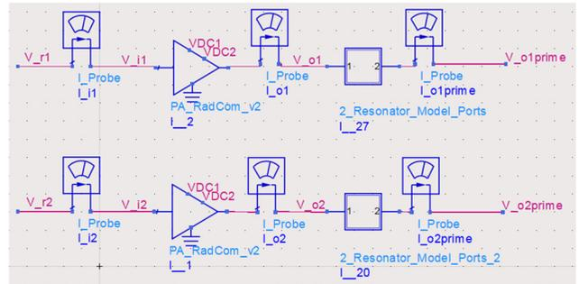
Fig. 2. Two of the 16 transmit chains used for simulation.
