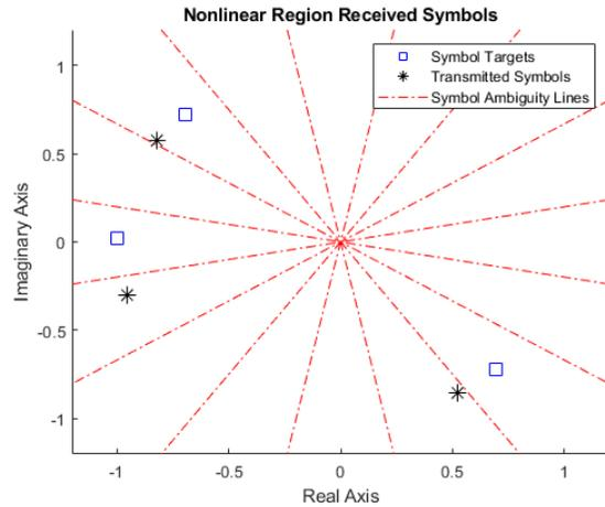
Fig. 13. The effect of nonlinear amplifier performance on the second set of communication symbols. In this test two symbols are transmitted incorrectly, namely the communication symbols in the  $-45^\circ$  and  $-60^\circ$  directions relative to boresight.
