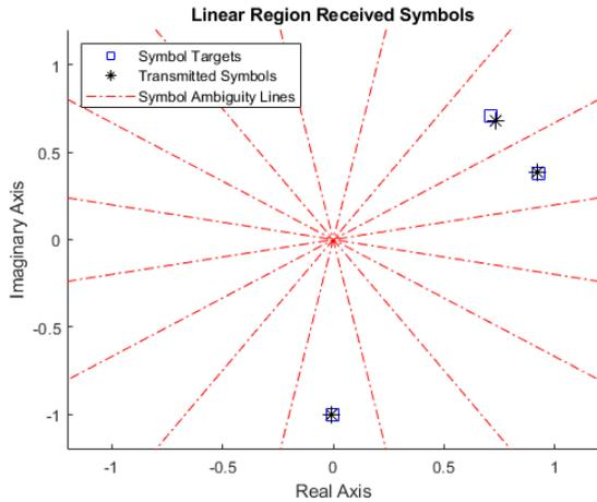
Fig. 7. Linear region communication symbol integrity. All symbols maintain integrity and are transmitted correctly.
