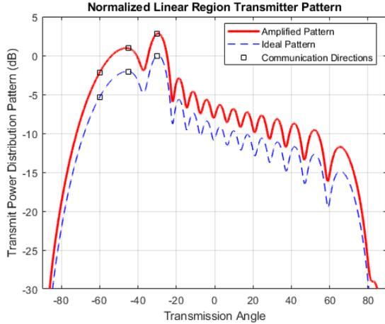
Fig. 10. Linear region amplifier effect on the transmission pattern including the second set of communication symbols. The linear region of the amplifiers reproduces the ideal pattern accurately.
