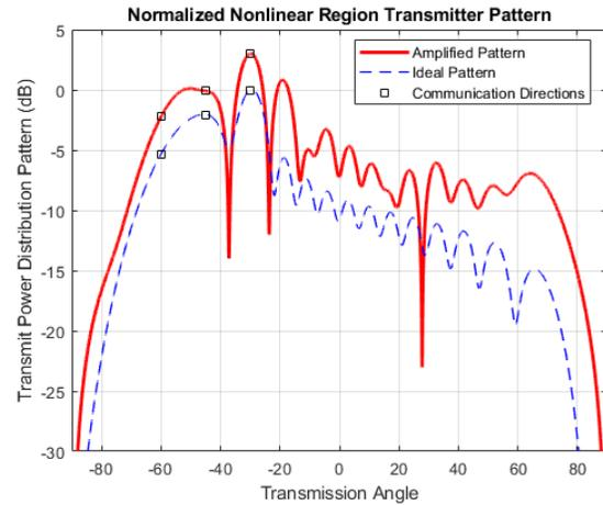
Fig. 12. Nonlinear amplifier effect on the transmission pattern for the second set of communication symbols. The transmission pattern does demonstrate distortion from the ideal pattern.
