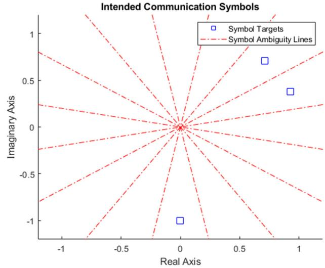
Fig. 5. Intended directionally modulated 16-PSK symbols. Because all symbol information is encoded in the phase of the transmission, all symbols are normalized to a magnitude of 1 for clarity. Dashed lines indicate the ambiguity angles for a 4-bit PSK with 16 possible symbols.
