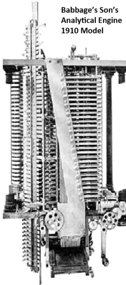
Fig. 1. Babbage Mechanical Computer – Babbage's 1837 Analytic Engine, was totally mechanical, and yet "Turing complete".
